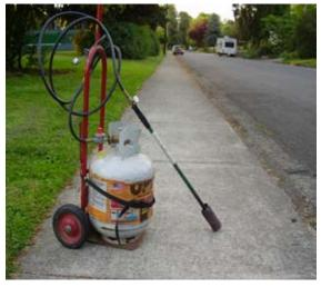
Propane-powered flame weeder attached to a dolly-mounted
